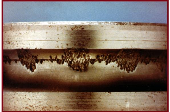
**Figure 1.** The damage shown here corresponds to the spacing of the rolling elements. The damage started as non-rotating vibration during shipping or storage.
